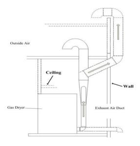
Figure 1. Typical Sectional View on Exhaust Duct Arrangement for Gas Dryer
