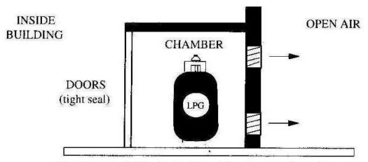
Chamber Located inside Building / Venting into Open Air
