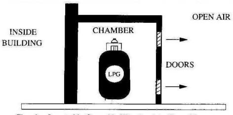
Chamber Located in Open Air / Venting into Open Air
