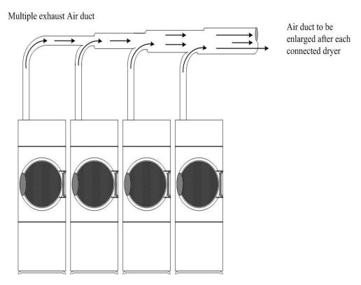
Figure 2. Typical Layout of Multiple Exhaust System
