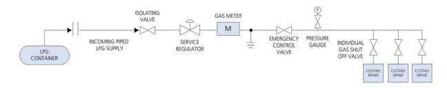
Figure 1 - A Typical Piped LPG Supply System For Gas Dryer
