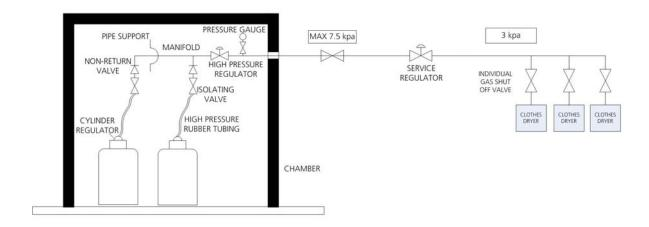
Figure 2(b). A Typical LPG Chamber Supply System (using High Pressure Regulator and Service Regulator) For Gas Dryer
