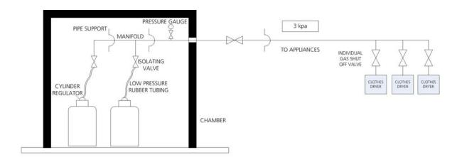
Figure 2(a). A Typical LPG Chamber Supply System (using Low Pressure Cylinder Regulators) For Gas Dryer
