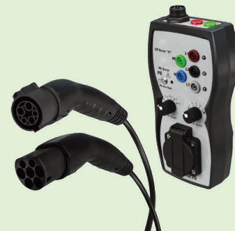
Test adapter for EV charging equipment
