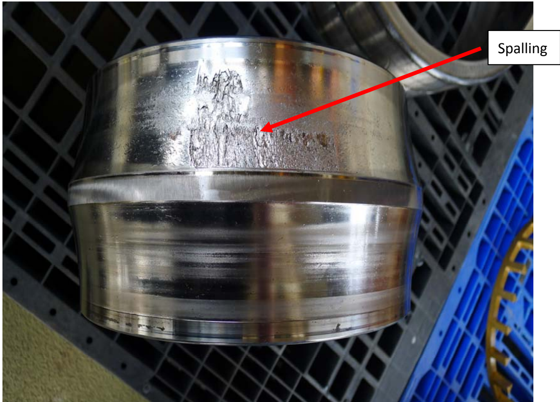
Figure 5: Spalling in the top raceway of the inner ring of the upper bearing
