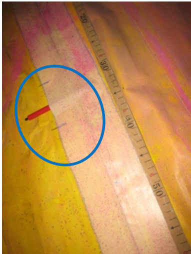
Figure 5a – Detachment in left covering strip at the edge (circled in blue)
