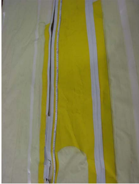
Figure 4 – Failure in right-hand rip panel joint (the orientation is reversed as viewed from inside of envelope)
