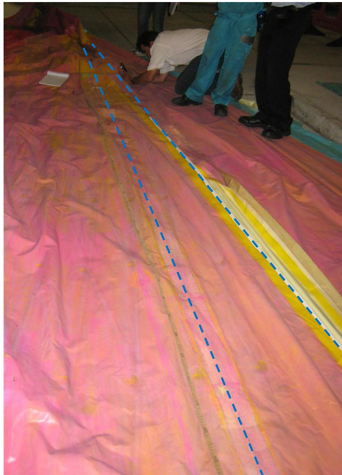
Figure A1 – Photo of the rip panel (rip panel joint indicated by dotted line)
