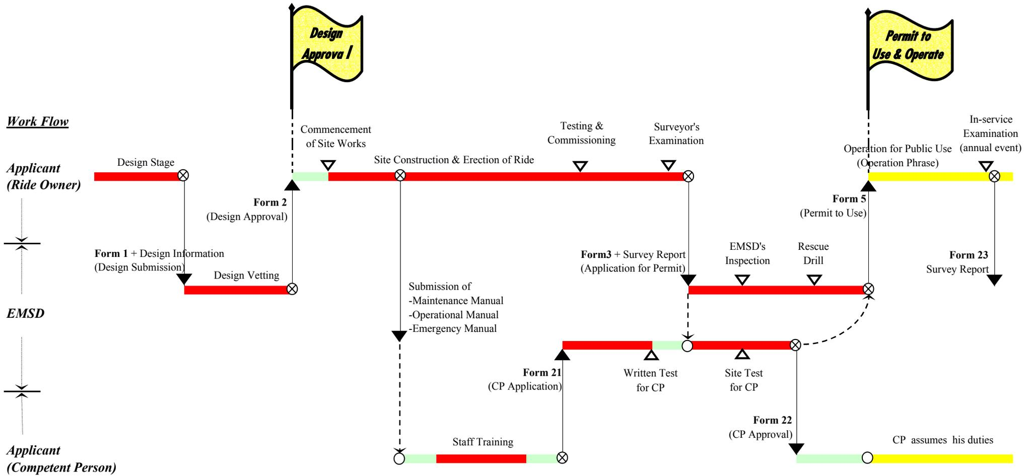
Figure 1 : Sequence of Events and Key Milestones for a Typical Licensing Process under Amusement Rides (Safety) Ordinance, Cap. 449
