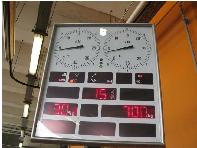
Brake Performance Shown on the Display of a Roller Brake Tester
