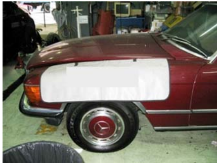
Cover the Front Fender with Protective Tape
