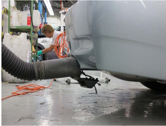
Guide the Exhaust from Vehicle to Outdoors via an Exhaust Hose
