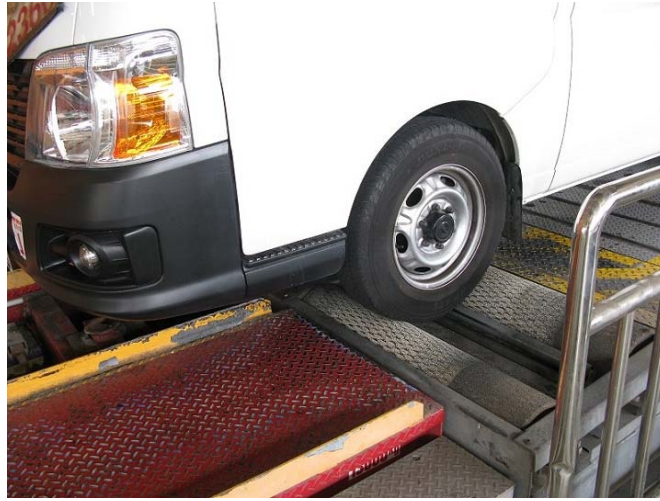
Position the front/rear wheels in the rollers
