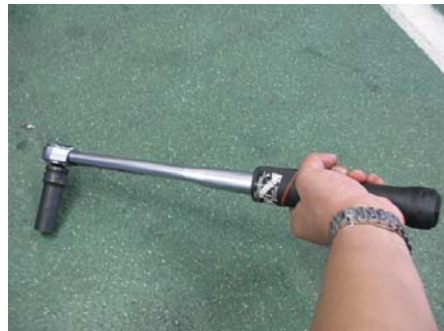
Set the Wrench by Turning the Handle
