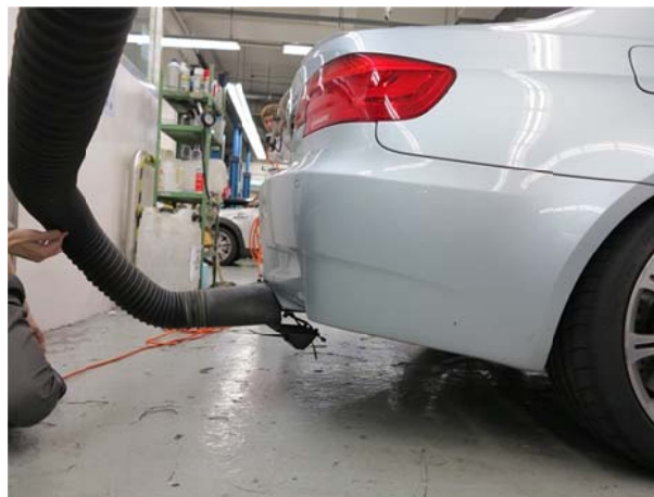
Guide the Exhaust from Vehicle to Outdoors via an Exhaust Hose
