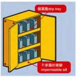
Designated place for storage of chemical waste, such as waste batteries and waste lubricating oil, etc.
