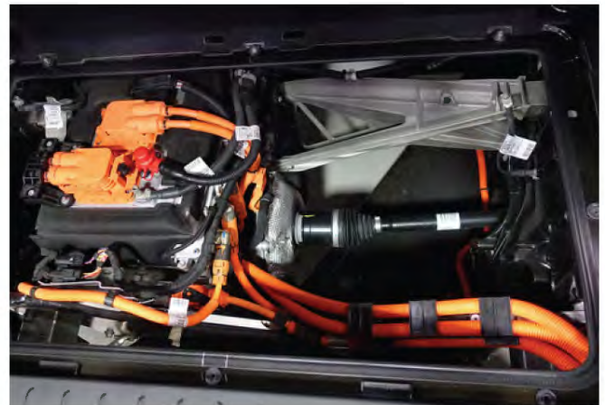
The orange wires in both EVs and HVs carry high-voltage power supply, and should not be disassembled on your own unless you have received specialised training
