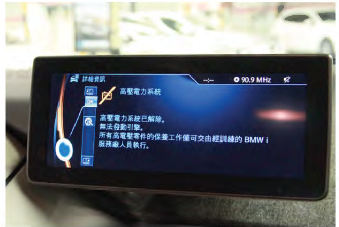
Confirmation displayed in the car after cutting off the power source
