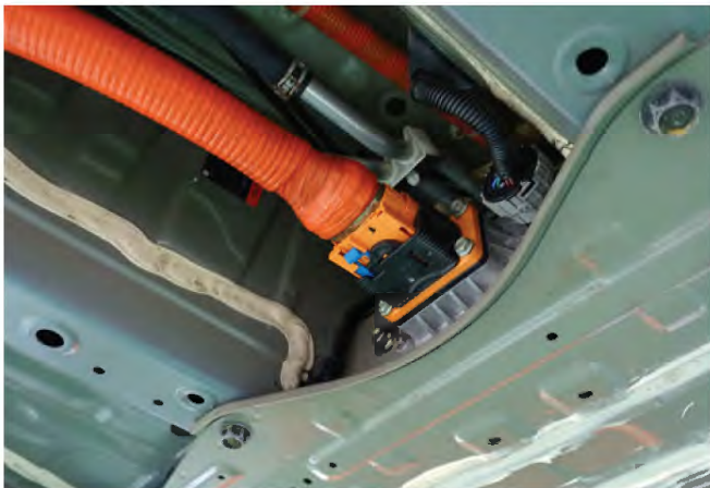
One of the high-voltage circuit breakers of a Japanese car model removes the service connector to cut off the high-voltage power source of the vehicle
