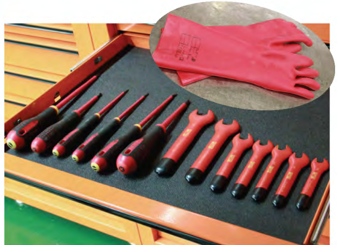
Use insulating gloves and insulating tools for maintenance to ensure safety
