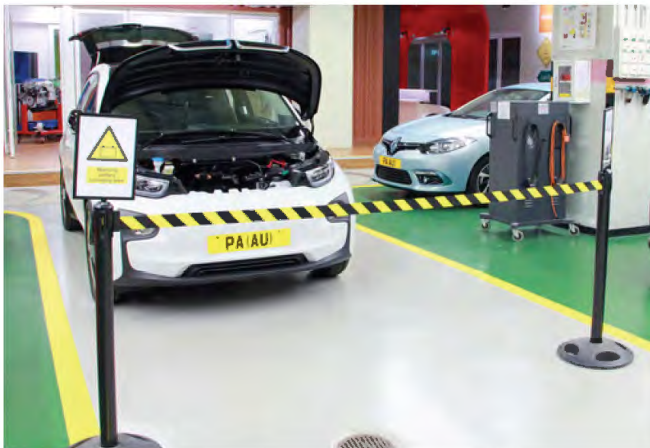
The area near the vehicle repair work must be fenced off with warning signs displayed
