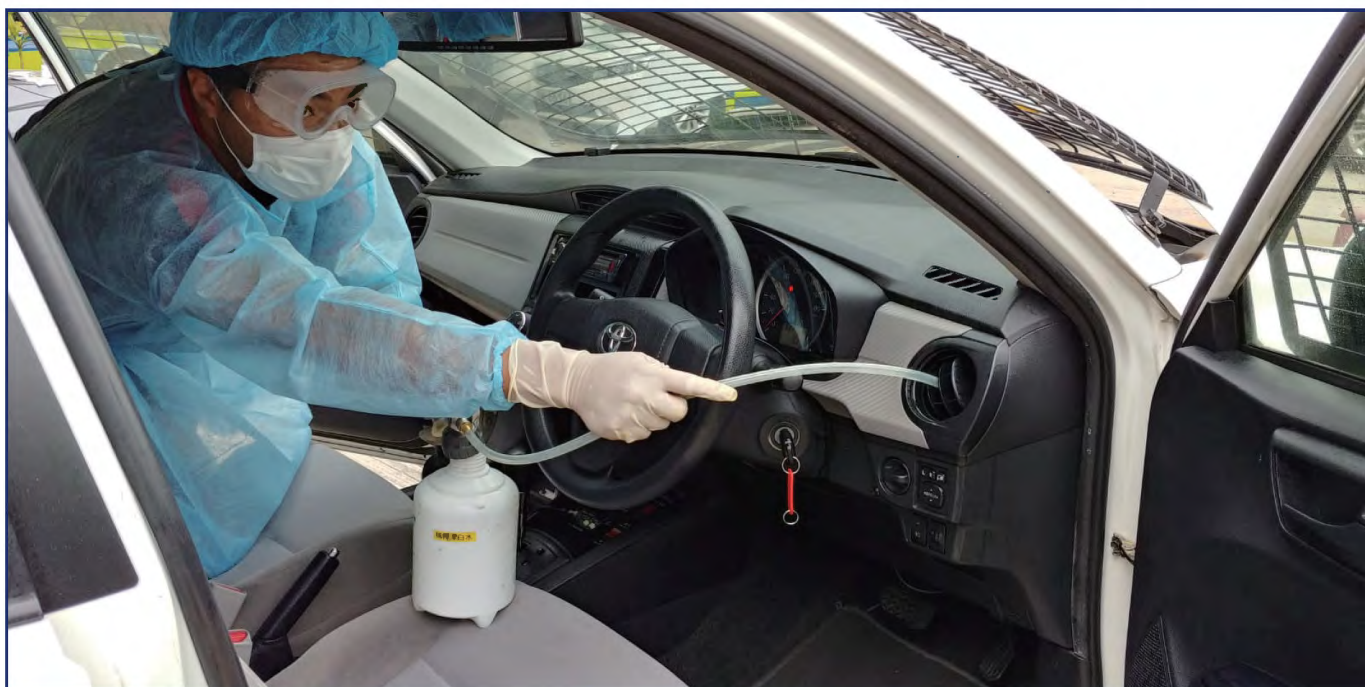
Spray condensers and air outlets with 1 in 49 diluted household bleach
