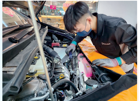
During the apprenticeship, Mr LEE Ling-hin learnt to use a testing instrument designed by the car manufacturer to shorten the time needed for fault finding.
