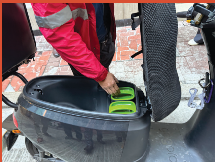
A rider demonstrated how to remove the battery from the EMC for charging.
