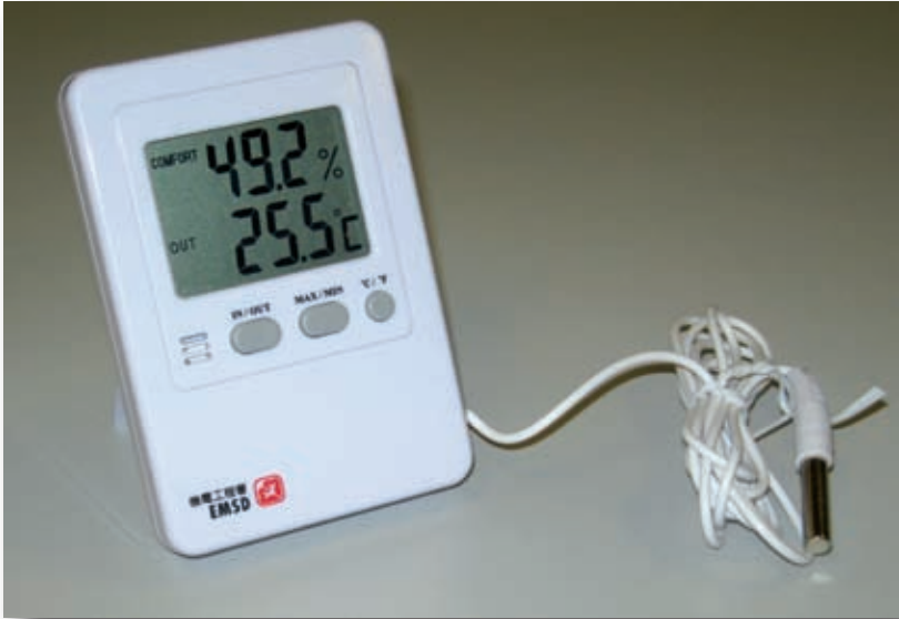
Fig 2. - A Digital Desktop Thermometer Provides More Accurate Visual Information About the Condition of Room.
