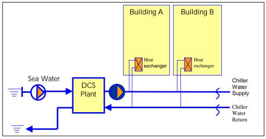
For a building served by District Cooling Scheme, its air conditioning system uses chilled fresh water produced by a central chiller plant for air-conditioning. Individual user buildings purchase chilled water from the DCS operator and do not need to install their own chiller plants. For this scheme, a central chiller plant, a pump house and a central distribution pipeline network are required.
