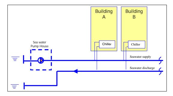
For a building served by Central Seawater Scheme, its air conditioning system uses seawater for cooling the chiller condenser. A dedicated central seawater supply system distributes seawater from the sea to the user building. The rejected warm seawater from the chiller condensers will be discharged to the sea through another dedicated outfall pipe. For this scheme, a central seawater pump house and a central distribution pipeline network are required.
