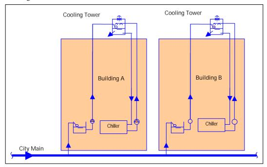
For a building adopting Cooling Tower Scheme, its air conditioning system uses an evaporative cooling tower for heat rejection. Water in the cooling tower will be lost due to the continuous evaporation, wind drift and bleed-off. The water lost will be replaced by water coming from city water mains. For this scheme, only city water main is used and no other infrastructure provisions are required.
