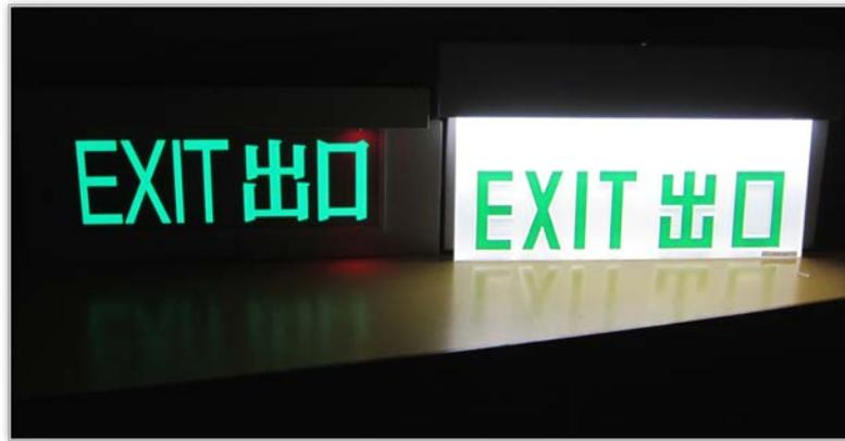
Figure 2 – Photo of tested LEC exit sign (left) and LED exit sign (right)
