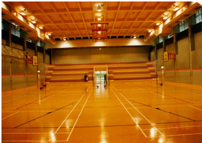
Fig.9: Reflective glare of HID lamps from floor surface
