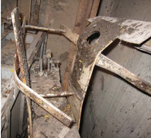
Figure 6A – Rope markings on counterweight pulley bracket.
