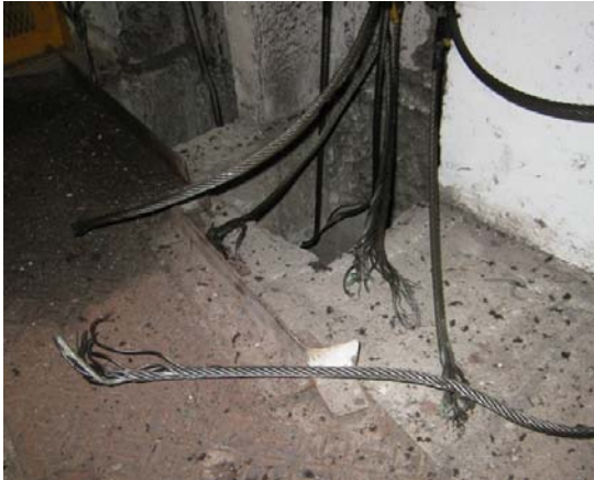
Figure 3 - Broken suspension ropes found in Lift Motor Room.
