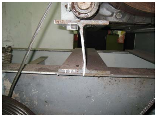
Figure 5B – Close-up view of the deformed I-beam.
