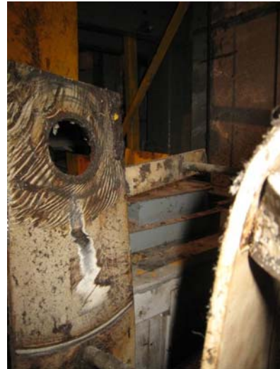
Figure 6B – Close-up view of the rope marks and pulley scratch mark on counterweight pulley bracket.
