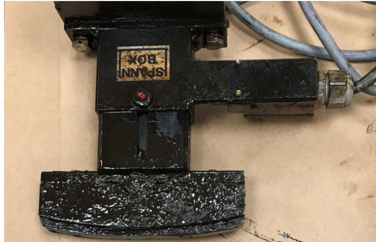
Figure 9: Photo of the BCD moving part and the shoe. Mixture of lubrication oil and dust formed the sticky grease, which was found on the surface.
