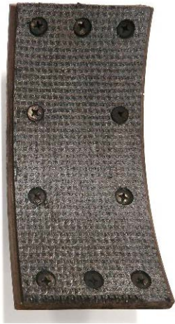
Figure 11: Right brake lining with all 10 mounting screws
