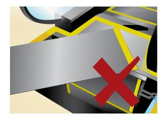
The guard is not properly installed
