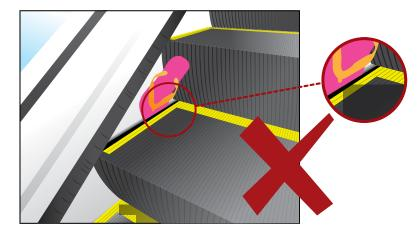
The clearance between the skirt panel and the step exceeds 4mm
