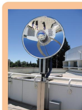
一座附有太陽追蹤器的太陽能照明系統能提高供電效率 An automatic sun tracking system is fitted to the hybrid solar lighting system to achieve a high collection efficiency
