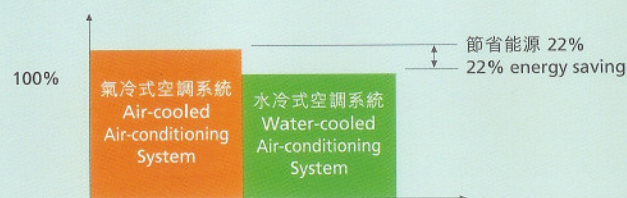
空調系統的能源消耗量 Energy Consumption of Air-conditioning System
