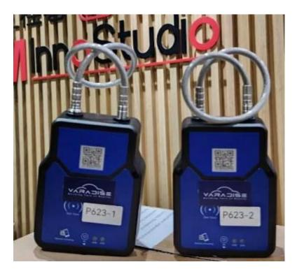
The Smart Locks used in the SSSS are designed for hazardous areas access control, such as electrical cabinets, lift fence doors, floor openings with latches, and confined space entrances. These locks are 4G-enabled and GPS trackable, providing enhanced security and monitoring capabilities.
