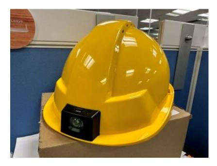
The Smart Helmets in the SSSS are equipped with 4G and GPS capabilities, along with sensors to monitor heart rate and body temperature. These helmets can detect free fall and standstill alerts, providing real-time data on environmental conditions and worker health. Built-in communication features facilitate instant communication between workers and safety managers, ensuring immediate warnings for potential hazards.
