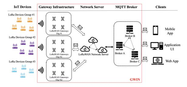
Fig. 2. The proposed LoRaWAN-based GWIN infrastructure
