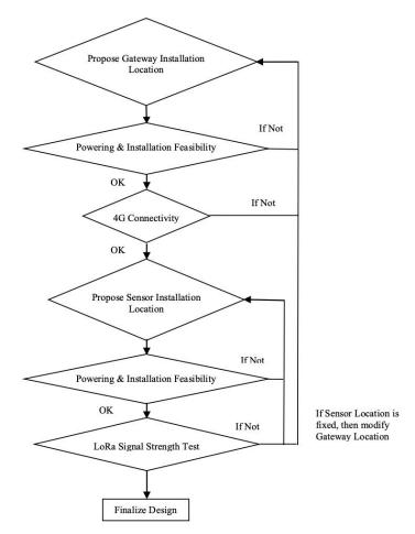
Fig. 15. Site survey test procedure
