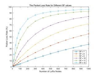
Fig. 41. The packet loss rate for different SF values (i.e. SF = 7,8,9,10,11,12) - 124 -
