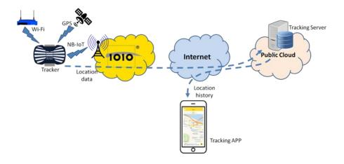
Fig. 8. GPS Tracker System Architecture
