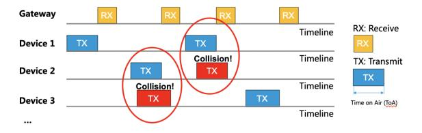
Fig. 36. Packet collision due to pure ALOHA scheme in LoRa network (End devices use same channel and same SF for transmission)
