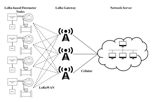
Fig. 24. LoRa-based flowmeter system structure
