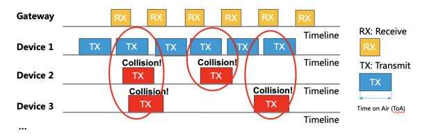
Fig. 37. Packet collision due to unreasonable resource allocation in LoRa network (End devices use same channel and same SF for transmission)
