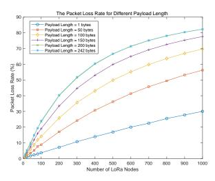
Fig. 42. The packet loss rate for different effective payload length (i.e. 1, 30, 50, 100, 150, 200, 242 bytes)
