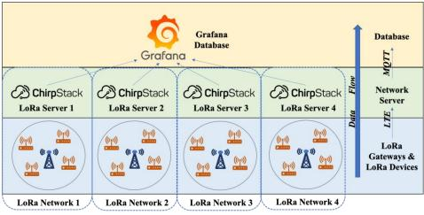
Fig. 40. The structure of four LoRa networks
