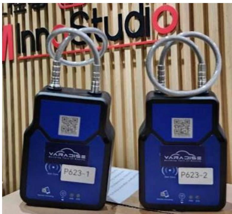
The Smart Locks used in the SSSS are designed for hazardous areas access control, such as electrical cabinets, lift fence doors, floor openings with latches, and confined space entrances. These locks are 4G-enabled and GPS trackable, providing enhanced security and monitoring capabilities.
