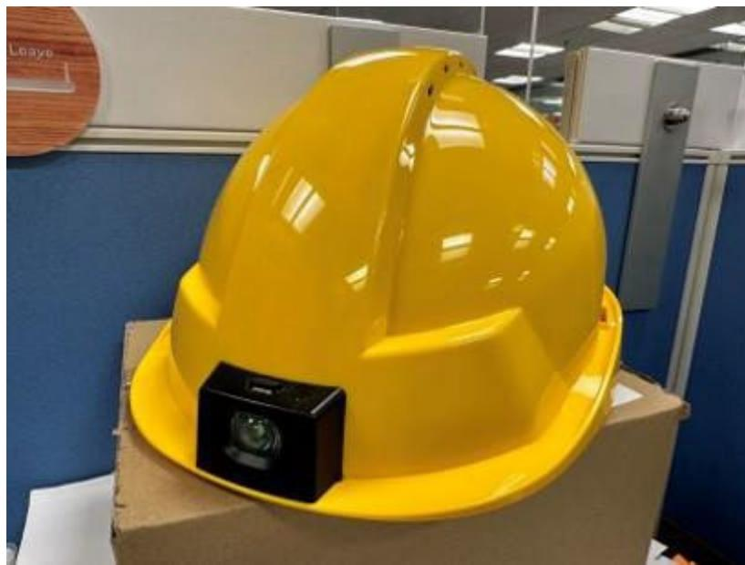
The Smart Helmets in the SSSS are equipped with 4G and GPS capabilities, along with sensors to monitor heart rate and body temperature. These helmets can detect free fall and standstill alerts, providing real-time data on environmental conditions and worker health. Built-in communication features facilitate instant communication between workers and safety managers, ensuring immediate warnings for potential hazards.
