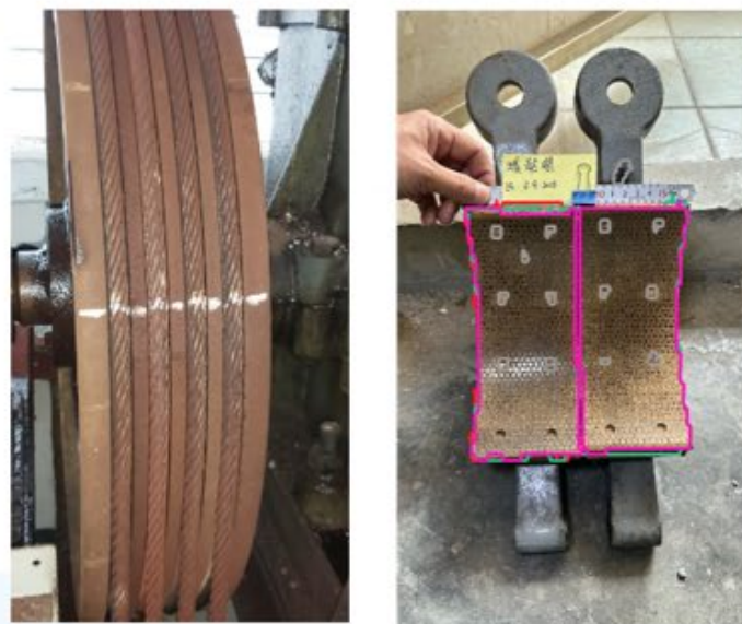
Brake Pad Cracks (light) Burnt Mark (light) Exposed Rivet Heads (severe) Excessive Wear (light)
