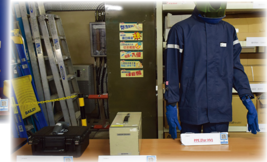
手提式局部放電檢測儀、真空開關絕緣測試儀及個人防護裝備 Ultra TEV Detector, Vacuum Checker and Personal Protection Equipment
