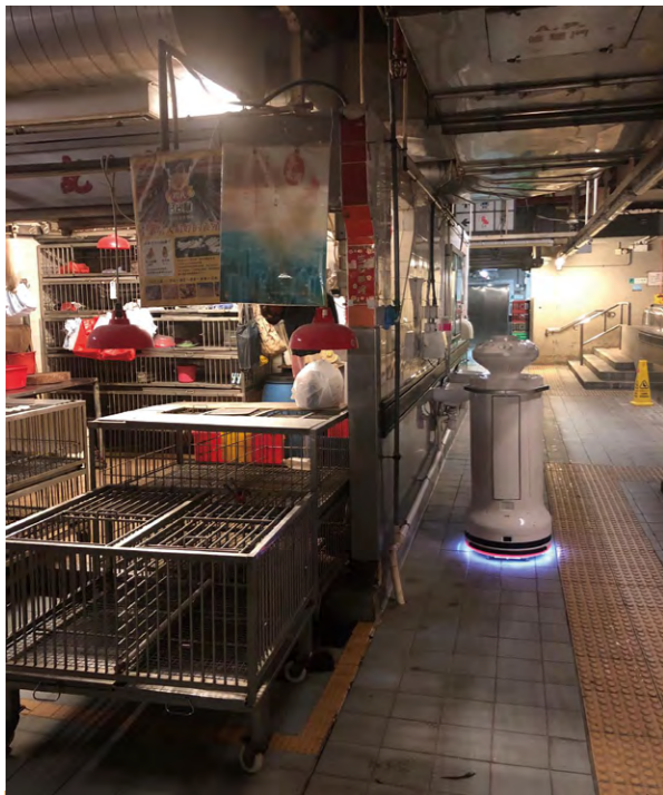
配備紫外線消毒燈的消毒機械人在公眾街市操作的情況 A disinfecting robot equipped with UV lights operates in a public market.
