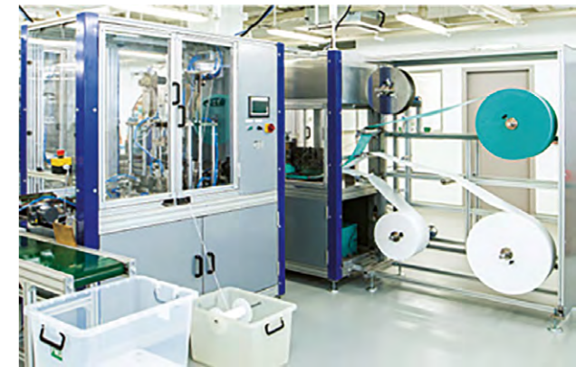
懲教署近日投產的全自動口罩生產機 The CSD's fully automatic mask production machines have been recently put into operation
