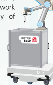
首個檢疫樣本收集機械人的概念驗證 Proof-of-concept of the first robot for specimen collection and delivery
