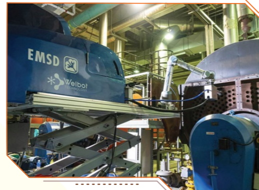
智能鍋爐維護機械人是機電署取得金獎的項目之一 The Smart Boiler Servicing Robot is one of the EMSD's gold medal projects
