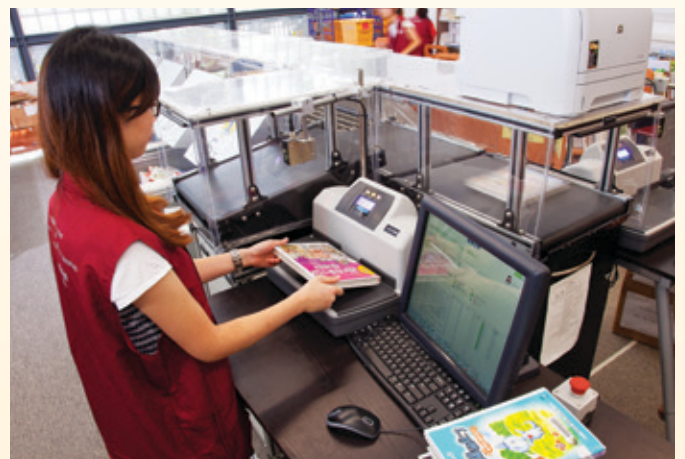
屏山天水圍公共圖書館職員正在使用書籍分揀系統分揀書籍。系統根據電腦條碼將書籍按類別放進不同的箱子。 A librarian at the Ping Shan Tin Shui Wai Public Library is using the book sorting machine. Using bar codes, the machine will sort books into different boxes according to the category of each book.
