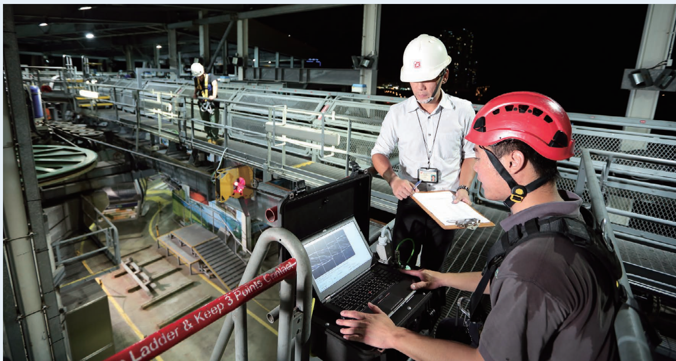
(上下兩圖) 機電工程署人員測試昂坪360的新「牽引纜自動檢查系統」：系統會使牽引纜檢查工作更準確、更有效率。 (Both photos) EMSD officers testing the new Automatic Haul Rope Examination System in Ngong Ping 360. The system will make the haul rope inspection process more accurate and efficient.
