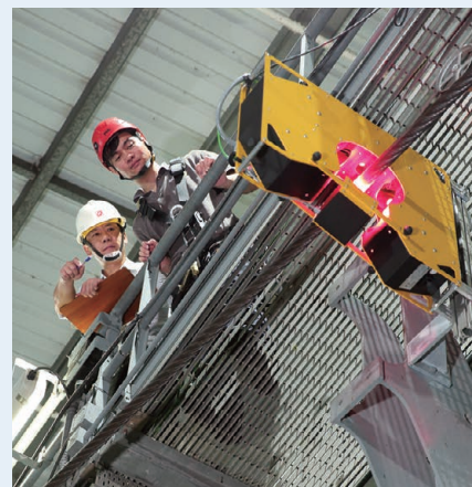
(上下兩圖) 機電工程署人員測試昂坪360的新「牽引纜自動檢查系統」：系統會使牽引纜檢查工作更準確、更有效率。 (Both photos) EMSD officers testing the new Automatic Haul Rope Examination System in Ngong Ping 360. The system will make the haul rope inspection process more accurate and efficient.
