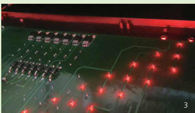
我們替運輸署更換行車線管制燈號和可變車速限制標誌，從而提供更好的訊號顯示，以確保青馬管制區的行車安全。以上1-4照片分別為舊式鎢鹵燈；新式發光二極管燈；新式發光二極管燈內部及青馬管制區的行車線管制燈號。 We assisted Transport Department in replacing the LCS and VLSL to provide a better display of signals in order to ensure road safety in TMCA. Photos 1-4 above show the old Halogen lamp type; the new LED type equipment; the internal of new LED type equipment; and LCS equipment at TMCA, respectively.
