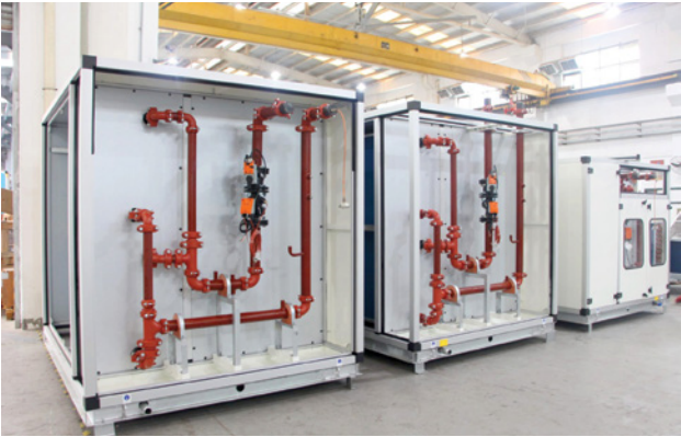
啟德區域供冷系統三號廠房應用了機電裝備合成法，大部分複雜組件都在工廠預製，再於工地裝嵌。這不但加快工程進度，也可避免工程人員在狹窄環境中工作的潛在安全問題。 The Kai Tak DCS Plant No.3 applied the MiMEP method. Most of the complex components were pre-assembled in factories and then assembled at the construction site. This not only accelerated the progress of works, but also avoided potential safety hazards to engineering personnel in cramped working environments.
