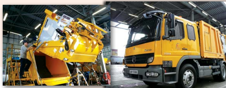
「歐盟五期」環保垃圾收集車，除了加強減排之外，其垃圾儲存間更完全密封，可盡量阻隔臭味。 The environmentally friendly "Euro V" refuse collection vehicles achieve cleaner emission while odour is minimised with the use of the enclosed refuse storage compartment.
