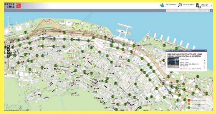
以地理資訊系統為基礎的遙距監測系統,裝置了多個操作界面,方便進行資產管理工作。上圖的用戶介面顯示各交通燈的位置和狀況。 In the GIS-based Remote Monitoring System, multi-operational layers have been implemented to facilitate asset management activities The above user interfaces show the locations and healthiness of various traffic lights.
