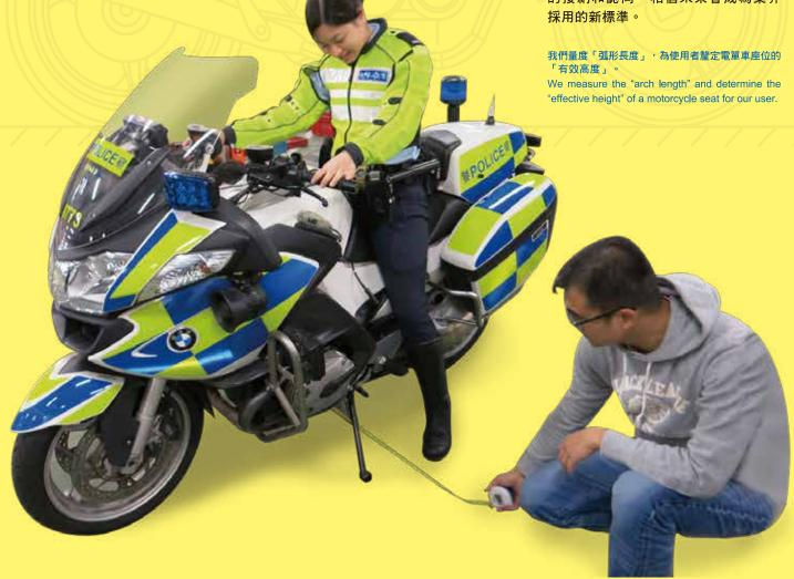
Our initiative to establish an "effective height" of a motorcycle seat by re-defining and standardising the measuring method will help enhance the occupational safety and health (OSH) of users. The new motorcycle seat height standard and measuring method have been well received by client departments, users and the trade.
