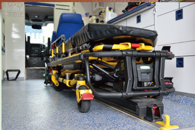
救護車內的電動升降救護車床處於鎖定狀態。 The stretcher is in locked status on ambulance.
