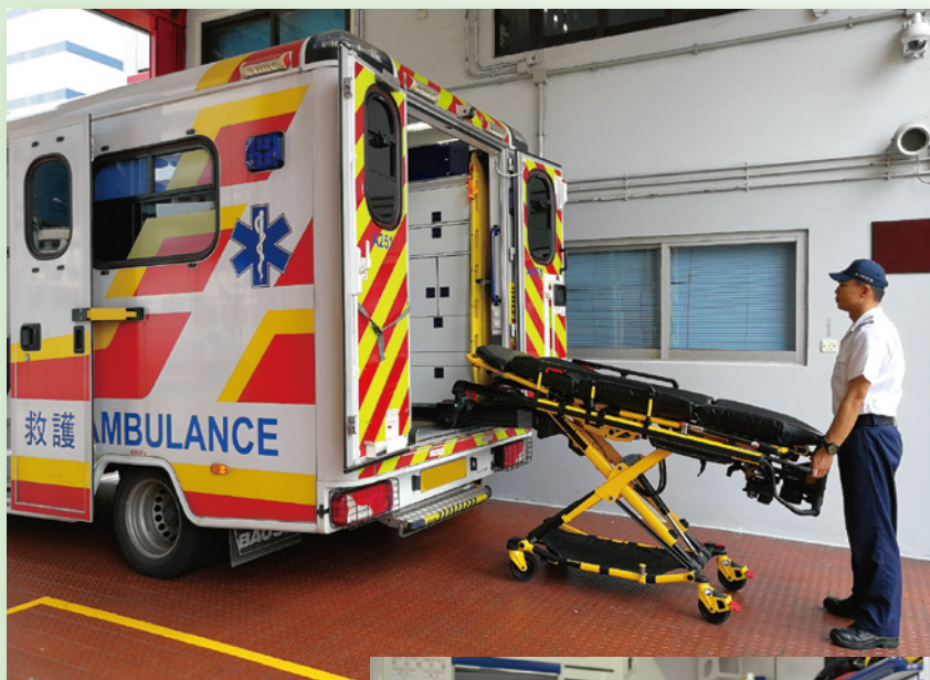
◀ ▼ 電動升降救護車床腳摺合及進入救護車。 Powered stretcher is retracted and being loaded on ambulance.
