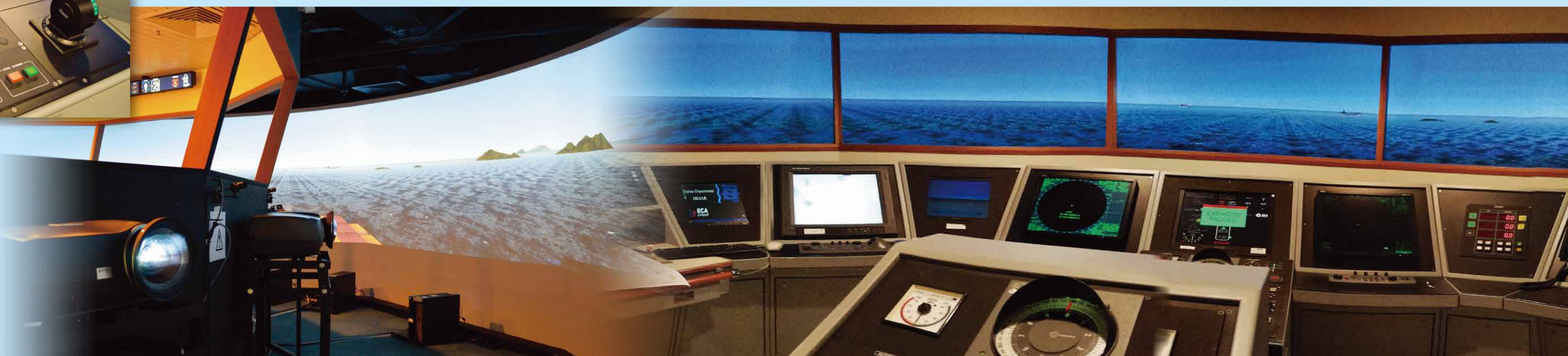
一號訓練駕駛台：船舶模擬器透過軟件控制七台投影機，投射出210度視角的無縫接合外景影像，讓駕駛台的學員仿如在真實的海洋環境中駕駛。 Full Mission Bridge 1: The seven projectors controlled by the simulator via its software project 210-degree seamless panoramic images, giving trainees at the bridge an immersive sailing experience.
