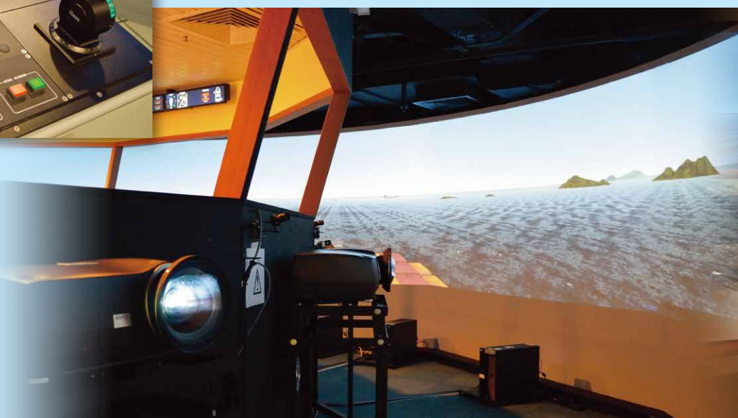
一號訓練駕駛台：船舶模擬器透過軟件控制七台投影機，投射出210度視角的無縫接合外景影像，讓駕駛台的學員仿如在真實的海洋環境中駕駛。 Full Mission Bridge 1: The seven projectors controlled by the simulator via its software project 210-degree seamless panoramic images, giving trainees at the bridge an immersive sailing experience.
