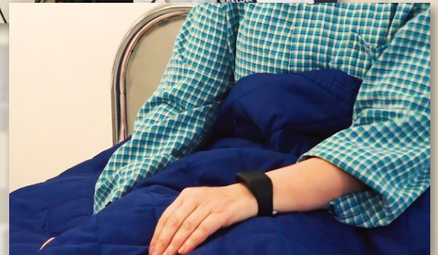
智慧手帶可監察在囚人士的心跳率、血含氧量等維生指標，以及他們所處的位置。 Smart wristbands can monitor such health signs as the heart rates and blood oxygen levels of persons in custody as well as their locations.
