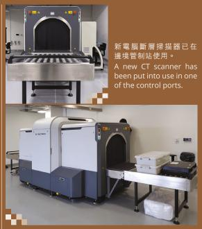
新設備可360度掃描物件,並以三維影像呈現掃描結果。 The new equipment can scan objects from 360 degrees and present the scanning results with 3D images.
